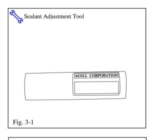
**NOTE:** The adjustment tool can be used if sealant is close to the door's edge. This must be done to allow for proper **Door Edge Guard** installation (Fig. 3-1).
